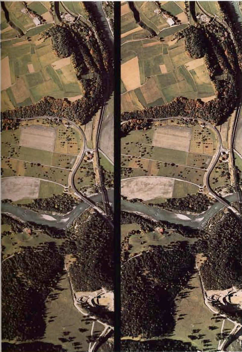
Color stereopair of Bonaduz, Canton of Grisons, Switzerland, October, 1975, photographs taken with Wild Leitz aerial camera RC10. Scale about 1:11,000.
